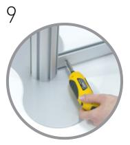
Connect the bottom horizontal rail to the two posts and tighten grub screws as before. Leave top rail until all verticals are in place. They will balance.
