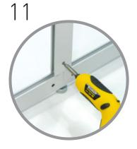
Connect middle rail(s)\* to the bottom rail and tighten grub screws. The middle rails have ta double graphic fitting strip on them. They will balance.
