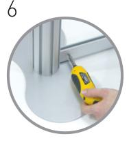
Connect first horizontal rails at the bottom of posts, leaving a 10mm gap between underside of rail and surface of base plate. Tighten clamp screws to secure in place.
