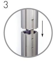
Join posts and tighten the grub screws to make assembly secure. Repeat for other base post.
