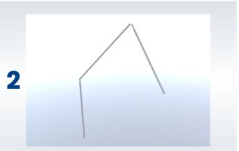
Unfold the 3-part supporting rod. Make sure that the parts click in each other.
